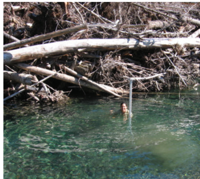
Thalweg depth decreased over 2 feet on average through the project reach. Scour at this structure was 7.2 feet. Photos credit: US Forest Service
