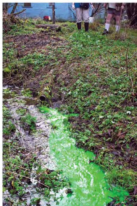
GREEN DYE IS USED TO REVEAL A FAILING SEPTIC SYSTEM
