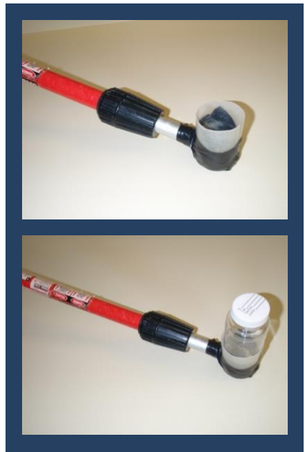
Figure 1: Sampling wand, made from an extendable paint pole with a cut Nalgene bottle attached at the end with electrical tape. Holds a 100ml sample bottle.
