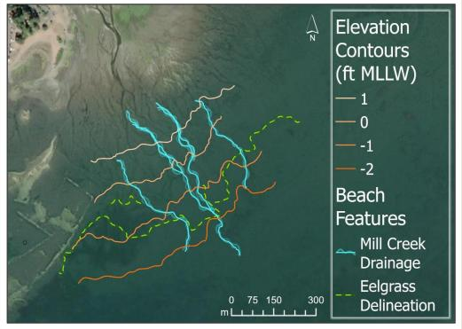
Figure 22. Map depicting the results of empirical feature mapping on the Big Mission Creek alluvial tideland area near Belfair State Park on June 25, 2021, including elevation contours (orange: lighter = higher elevation, darker = lower elevation), drainage channels (blue lines), and the shallow eelgrass delineation (green dotted lines).
