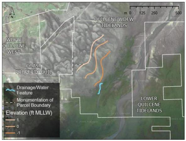
**Figure 14.** Map depicting results of empirical feature mapping at the head of Quilcene Bay on June 24, 2021, including elevation contours (orange: lighter = higher elevation, darker = lower elevation), drainage channels (blue lines), and on-beach monumentation line indicating parcel boundary (white dotted lines). Solid white lines indicate boundaries associated with a Beach Identification Number (BIDN) layer (WDFW 2021), and beaches are labeled by name.
